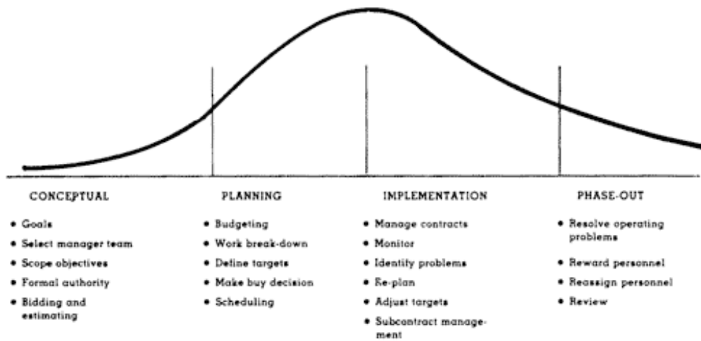
Figure 4: Cavendish and Martin's contract project life span
