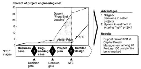
Figure 13: Abitibi's front-end loading of project development
