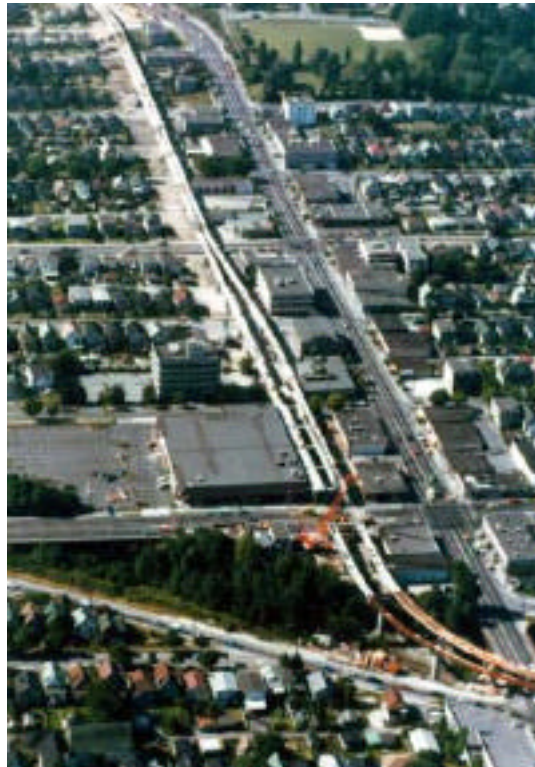
Aerial view shows major acquisition of property and track relocation to meet local opposition to running through a commercial center
